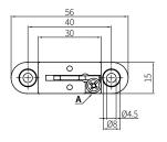
When installing the switch on a hinged door, turn the angle adjustment screw to adjust the inclination of the control key toward the door hinge.
