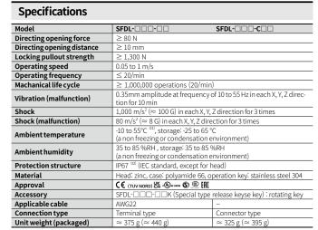
01) UL approved ambient temperature: 50°C 02) Rated protection structure is for the switch body. Be cautious about preventing the head part from entering the foreign
