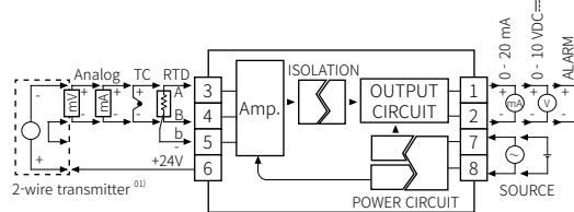
01) When using 2-wire transmitter, short between no.4 and 5 terminals.
