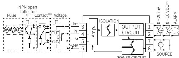
01) Connect external resistance  $10\text{ k}\Omega$  ( $\geq 1/2\text{W}$ ) to no.3 and 6 terminals for NPN open collector input.
