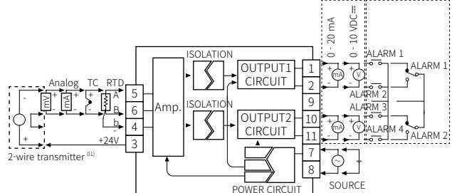
01) When using 2-wire transmitter, short between no.4 and 6 terminals.
