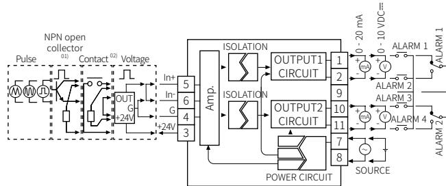
01) Connect external resistance  $10\text{ k}\Omega$  ( $\geq 1/2\text{W}$ ) to no.3 and 6 terminals for NPN open collector input.
