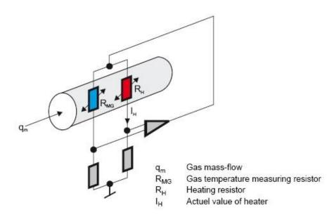
According to King's law, the heating power P, the temperature difference  $\Delta T$  (TRH-TRMG) and the mass flow rate are mathematical related. P/ $\triangle T$ =K1+K2 f(Q)K3 , the K1  $\times$  K2  $\times$  K3 are constants related to the properties of the gas. The flow meter is designed base on constant power measuring method, thus the RTD is heated in a consistent power and
